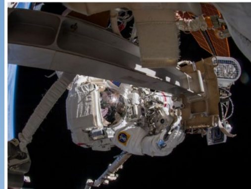
Figure 1: NASA astronaut Raja Chari connects an Ethernet cable to a wireless high-definition camera assembly on the main truss of the International Space Station, converting it to operate as a Wi-Fi access point. (Source: NASA)
